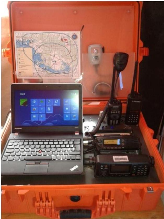
Picture 5: Portable radio communications set
