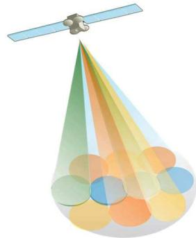
Picture 3: New generation footprint, Multi-beam architecture, Optimized for IP applications
